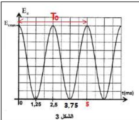
$$I_m = \sqrt{\frac{2E_{e max}}{L}} \quad \text{أي } I_m^2 = \frac{2E_{e max}}{L} \quad \text{ومنه } E_T = E_{e max} = \frac{1}{2} \cdot L \cdot I_m^2$$
